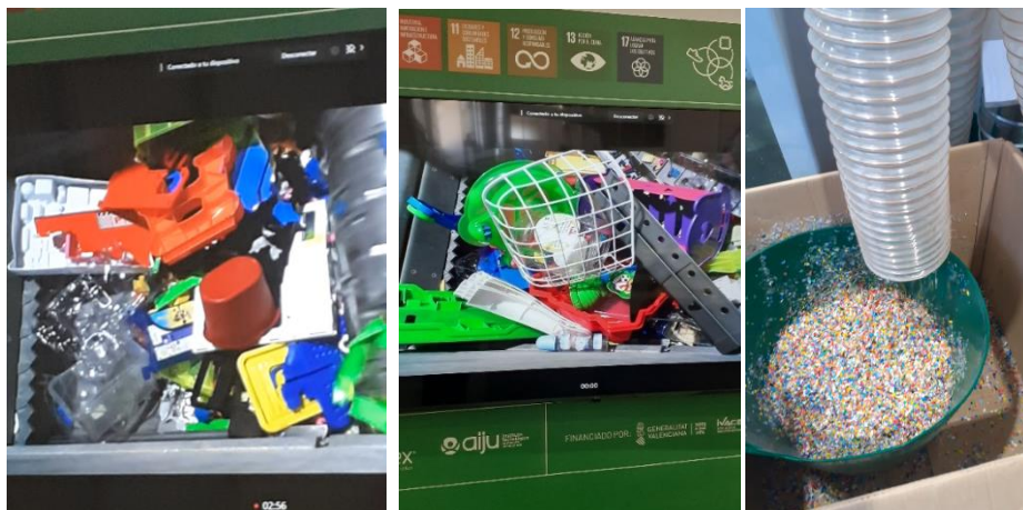
Figure 31. Grinding process and separation by flake size.
